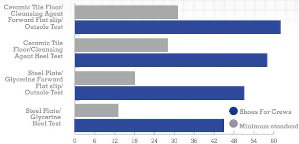
Slip Resistance Test EN ISO 13287:2012, performed by TUV Rheinland LGA Products GmbH in Leipzig, Germany during August 2018\* On a scale where 0.0 is the absence of friction and 1.0 is very high friction (e.g. dry carpet), SFC rated .63 - more than tripling the .18 minimum standard. All SFC shoes use the Shoes For Crews patented slip-resistant outsole. Product tested: BRIDGETOWN 28740
