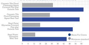
Slip Resistance Test EN ISO 13287:2012, performed by TUV Rheinland LGA Products GmbH in Leipzig, Germany during August 2018\* On a scale where 0.0 is the absence of friction and 1.0 is very high friction (e.g. dry carpet), SFC rated. 8.3 – more than tripling the .18 minimum standard. All SFC shoes use the Shoes For Crews patented slip-resistant outsole. Product tested:BRIDGETOWN 28740
